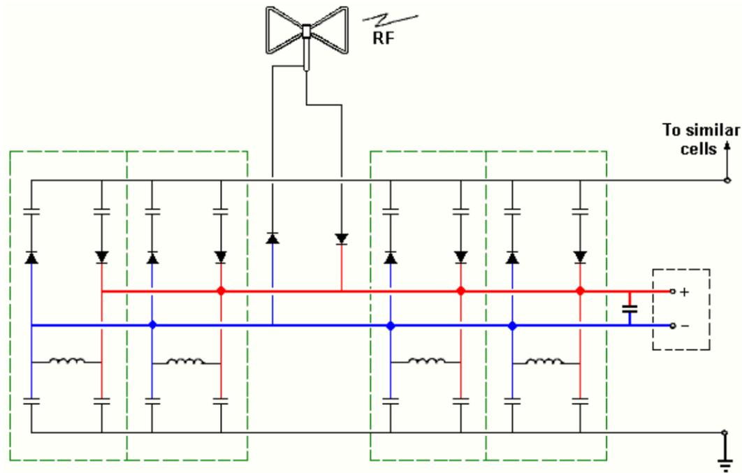
In one implementation of the invention this circuit is duplicated for each positive and negative output line. In another the circuit is coupled to additional identical circuits in order to increase the direct current output of the arrangement. In another implementation, the antenna used is a dipolar antenna of aluminium wire arranged in a "butterfly" configuration.
