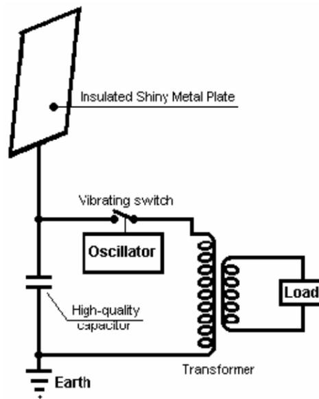
This system of Tesla’s picks up energy day and night. The capacitor gets charged up and a vibrating switch repeatedly discharges the capacitor into the step-down transformer. The transformer lowers the voltage and raises the current available and the output is then used to power the electrical load.
