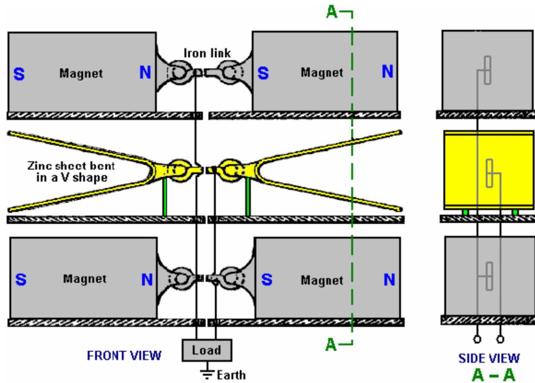
The zinc acts more effectively if installed as sheets bent into a V shape. The magnets and zinc sheets can be stacked vertically and/or horizontally and the greater the number used, the greater the electrical output. A good earth connection is recommended and presumably, the average cold water pipe of any house provides a more than adequate earth connection which is convenient to use, provided the pipework is made of metal.
